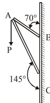
Suppose the force is  $\vec{P}$  resolved parallel to the arms AB and AC of the frame. The magnitude of the resolved component along the arm AC is  $x \text{ N}$ . The value of  $x$ , to the nearest integer, is \_\_\_\_\_.
