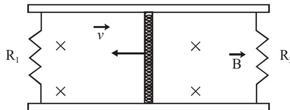
Two resistors  $R_1$  and  $R_2$  are connected across the ends of the rails. There is a uniform magnetic field  $\vec{B}$  pointing into the page. An external agent pulls the bar to the left at a constant speed  $v$ .
