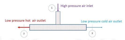
Assume constant specific heat of air is 1005 J/kg.K and gas constant is 287 J/kg.K. There is no work transfer across the boundary of this device. The rate of entropy generation is \_\_\_\_\_kW/K (round off to one decimal place).
