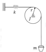
The pulley radius is r and its mass moment of inertia is J. Assume that the mass is vibrating harmonically about its static equilibrium position. The natural frequency of the system is
